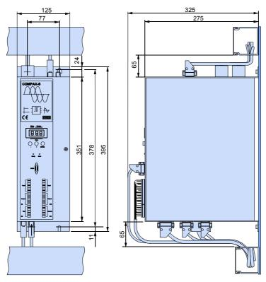
Fastening: 4 M5 hex-socket head screws Installation distance: 130mm (device distance:5mm)
